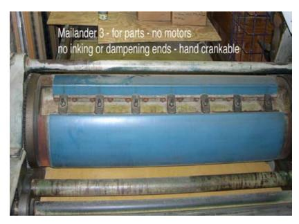
The third press is stripped of electric motors, as well as the inking and dampening ends. This is much smaller than the other two and lighter at about 4,000 pounds. It is a crankonly machine. Perfect for a student situation, no power to worry about. You could still run editions but you would have to hand dampen and hand ink. Peefect in an educational environment.
